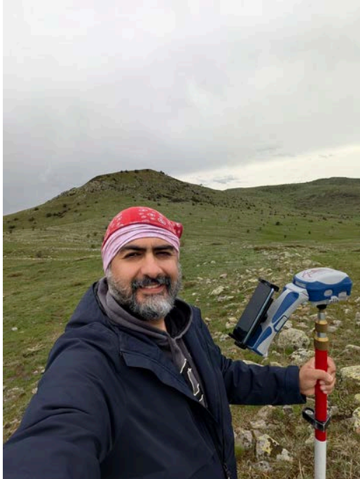
Photo of Atakan Atabas Conducting an electrical resistivity survey on a foggy, cold day in the field.
