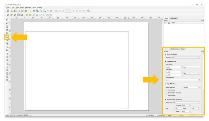
9. The map design can be adjusted through the **Item Properties** tab.
