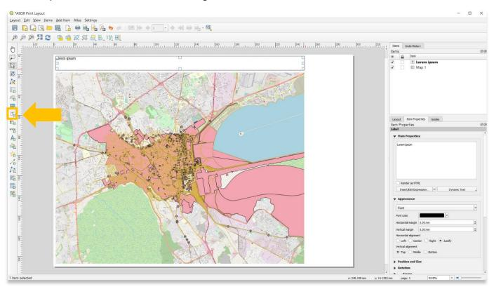
11. Label designs can be adjusted through the Item Properties tab.
