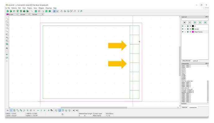
19. Add labels (text) to the Text block by first creating a new layer (0.25mm line width), then select the **MText** tool. Adjust the height, font, and alignment as needed.
