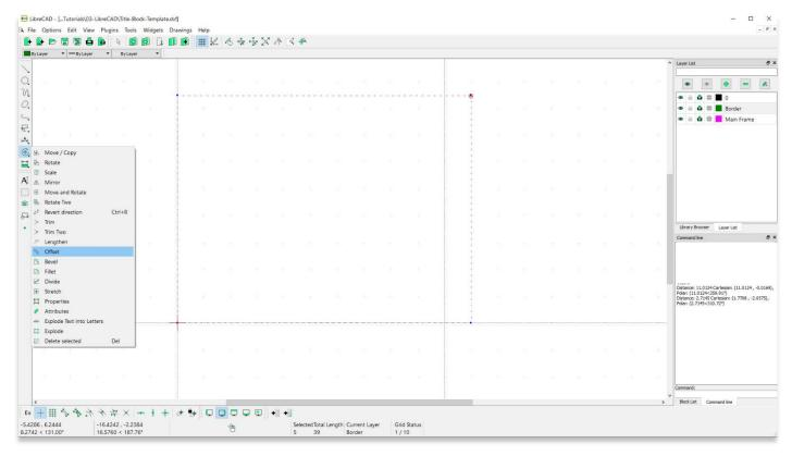
12. Move cursor within the rectangle. Type "0.3" in the Distance field. Click on mouse to place the offset drawing.
