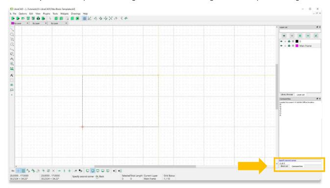
10. Create a new layer named, Border. Set the line width to 0.35mm.
