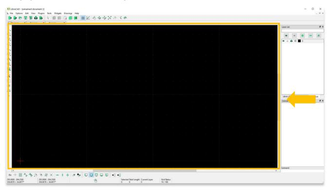
3. Before beginning a new project, turn on the **Grid** and check your **Grid Status**. By default, your **Grid Status** will be set to **10/100**. This means that the distance between each dot is 10mm and between each line is 100mm.
