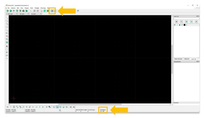
4. Unit measurements can be changed by selecting Current Drawing Preferences under the Options menu.
