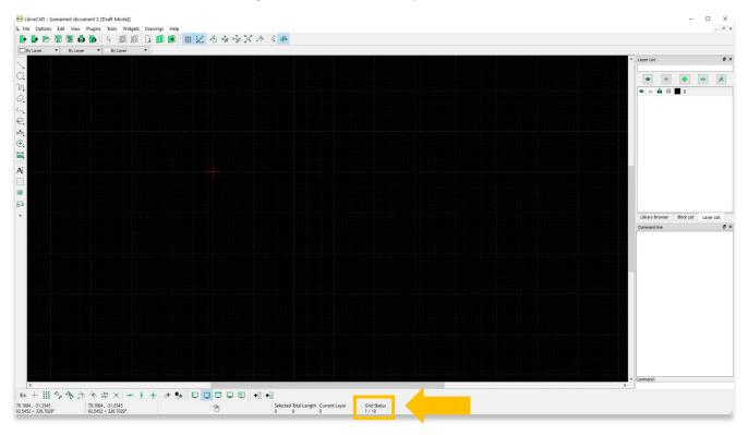
8. **Origin Point**: Everything drawn in LibreCAD is based on an X,Y coordinate system with an absolute origin or Zero point located at the red cross. Every feature that you draw is located in relation to this origin through X,Y coordinates.
