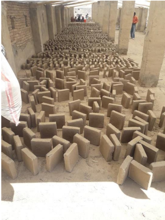
The ASOR CHI sponsored project to restart production at the Heraqla brickyard near Raqqa to produce appropriate, traditional bricks for the stabilization of the Raqqa Museum (ASOR CHI).
