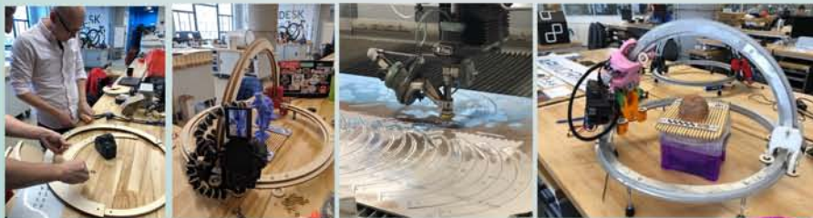
Start to finish digital imaging of Egyptian ushabti from the Brandeis CLARC; SCAPP scanning, processing in Agisoft Metashape and Reality Capture, final processing in Simplify3D for printing.
