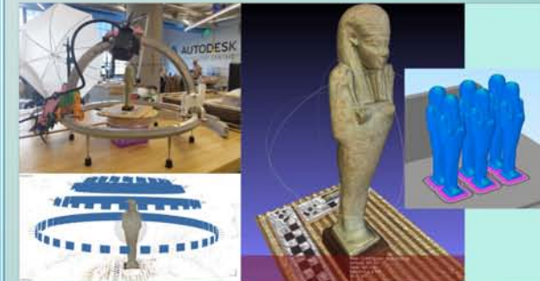
Start to finish digital imaging of Egyptian ushabti from the Brandeis CLARC; SCAPP scanning, processing in Agisoft Metashape and Reality Capture, final processing in Simplify3D for printing.
