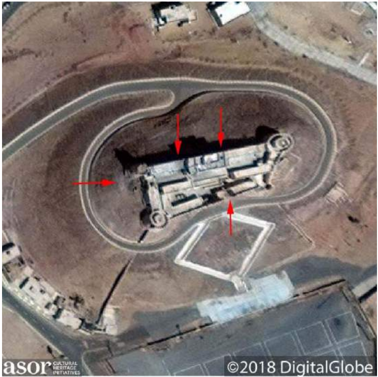
Sabha Castle with visible scorch marks, debris and a hole along the western and northern walls of the castle, as indicated by red arrows. There is also a possible breach in the southern wall (DigitalGlobe NextView License; March 9, 2018)
