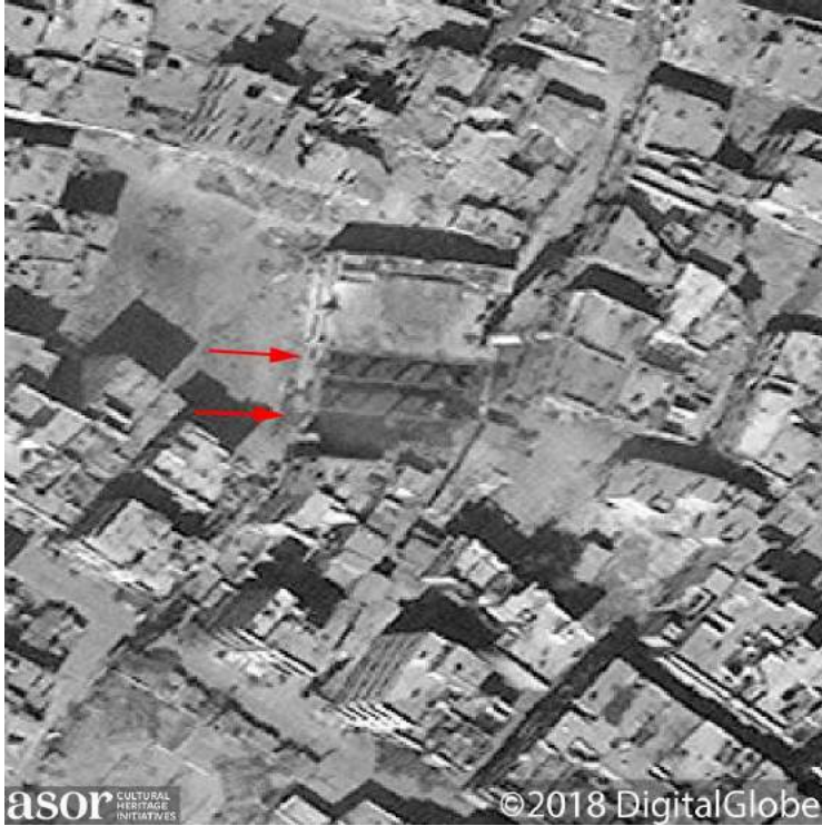
Red arrows indicate where the southern half of the roof of al-Kabir Mosque collapsed, exposing the interior pillars of the mosque. Smoke from the event is visible in the satellite image (DigitalGlobe NextView License; March 12, 2018)
