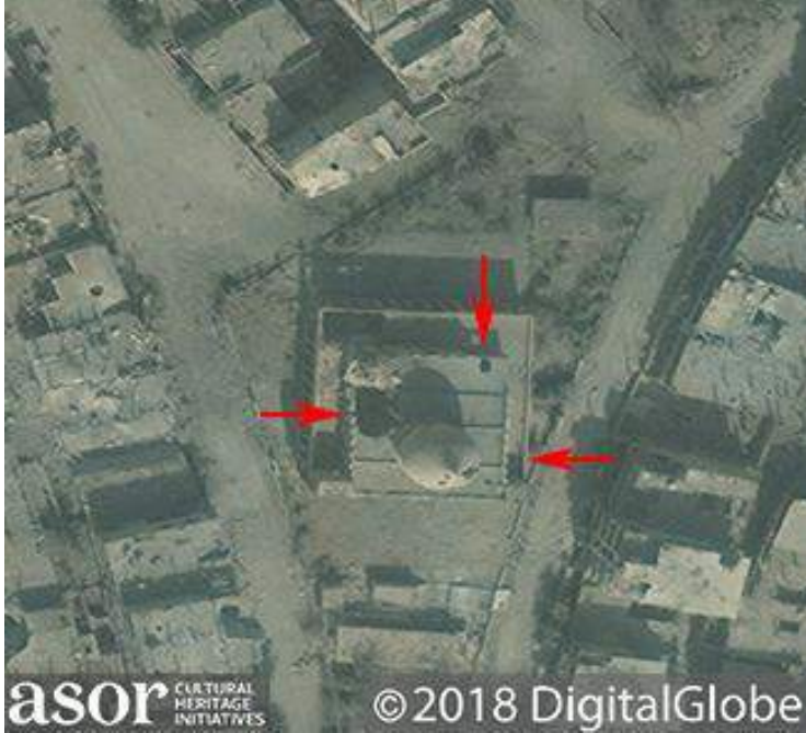
Multiple holes visible in Othman Bin Affan Mosque roof (DigitalGlobe NextView License; October 27, 2017)
