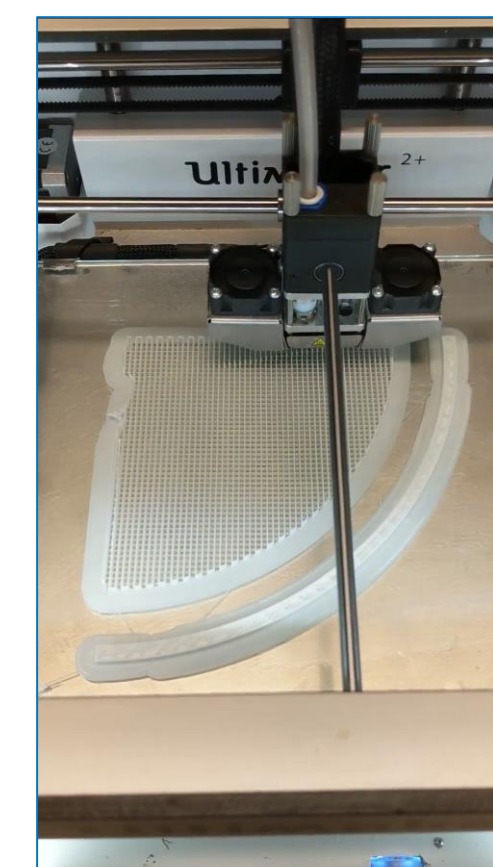
Figure 5, 6, & 7: 3D modelled Persian Period Mortaria with laser scanned original sherd (Left). 3D printed Persian Period Mortaria with original sherd (Middle), Section of a vessel being 3D printed on an Ultimaker 2+ (Right)
