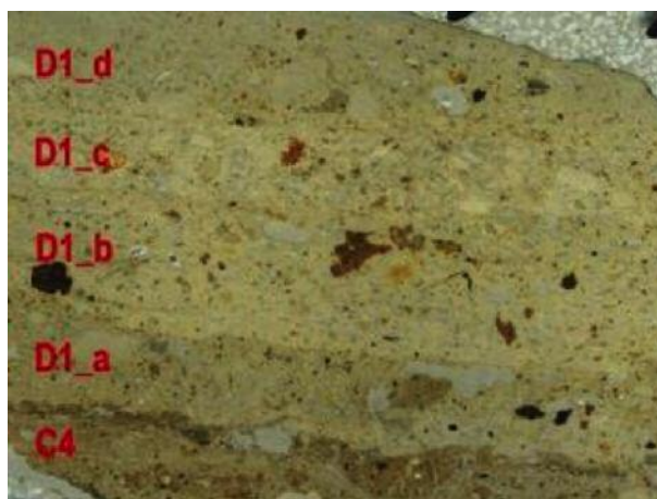
Fig. 12: (width of slide is 3.9 cm): Lime plaster fragment (sample MEG11Q-3, from Square H/6) that includes four consecutive layers, each ca. 0.5 cm thick. The plaster applications include coarse fragments of pottery, some surrounded by sedimentary rotational features, ash, burned compacted dung fragments, and phytoliths in pseudomorphic voids after chaff temper. Unreacted lime is present as well. The four layers differ in porosity, where in the more porous layers chambers exist as well as secondary sparitic calcite, indicating that porosity is secondary, due to dissolution.
